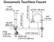
■Mounting deck thickness: 1/4" (5 mm) - 2" (50 mm) ■Spout hole: Ø1-1/4" (Ø32 mm) - Ø1-3/8" (Ø35 mm)
